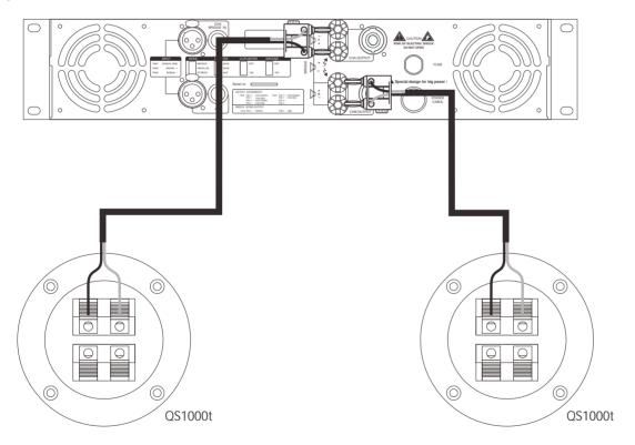
Attention: The impedance of connected speaker must match the impedance of amplifier output.
