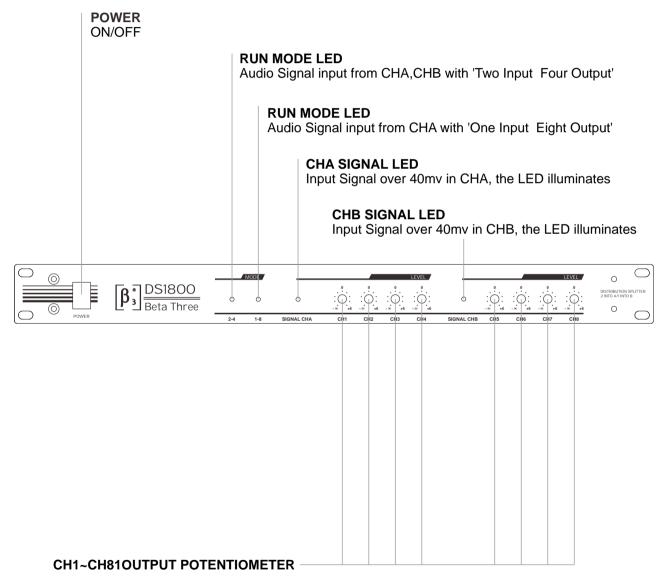
Signal output increasing gradually up to +6dB when turning the potentiometer in clockwise orientation. Signal output decreasing gradually up to no signal occurring when turning the potentiometer in anti-clockwise orientation.
