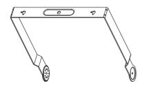
Warning: Make sure the mounting accessories safety factor not less than 5:1 or meet the local standard during installation.
