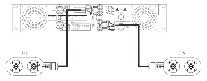
Attention: The impedance of connected speaker must match the impedance of amplifier output.
